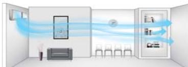
Press "Turbo" button on remote controller to enjoy a larger air flow, which enables the indoor temperature to reach the set temp in a shorter time.
