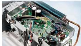
In the inverter outdoor unit, the PCB could work well even when temp is up to 85°C, and also metal casing is fire-proof.
