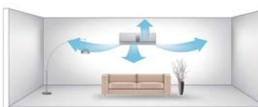
The louver can be vertically or horizontally adjusted so as to maximize comfort in the room.
