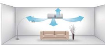
The louver can be vertically or horizontally adjusted so as to maximize comfort in the room.
